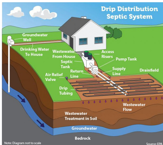
Figure 5. Diagram of a drip dispersal system. Wastewater is pumped from pumping chamber to drip tubes typically placed shallow in the soil.
