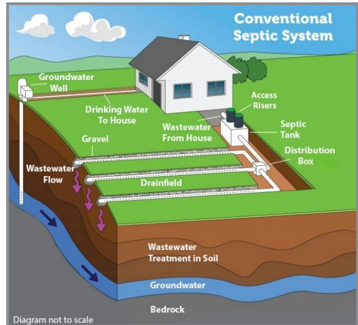
Figure 1. A conventional septic system with a tank, distribution box and drainfield showing the flow of wastewater including soil treatment and connection ultimately to groundwater. Source: EPA.
